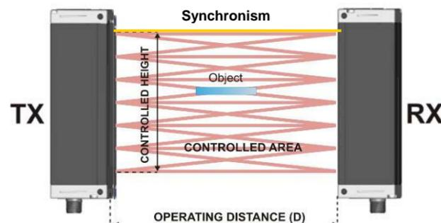
The beam interruption due to the passage of an object inside the controlled area causes the closing of the switching output and the variation of the device analogue output signal. Small objects can be detected (reaching dimensions of only 0.5 mm) and with a reduced surface area.
