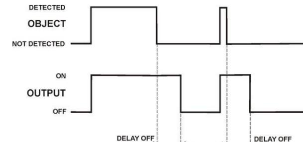
To set the DELAY OFF function select the "dIOF" text from the parameter menu.
