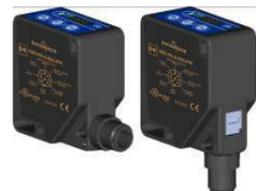
The M12 connector can be oriented at three different positions using the specific fastening spring and rotating the block of 180° until reaching the lock position. If the target to detect is very shiny (metal plate), we suggest to angle the sensor 5°-20° respect to the material to detect and the material movement direction.
