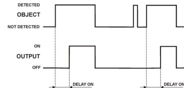
To set the DELAY ON function select in the menu parameters the "dOn" text.
