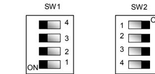
**NOTE:** configure the two dip-switch in the same way, otherwise the central control unit is locked and code '8' is *displayed*.
