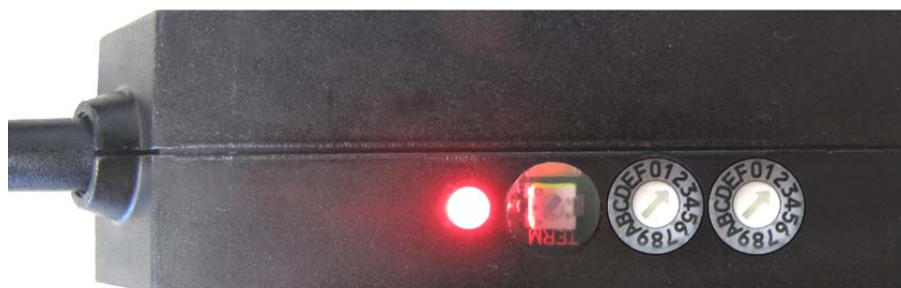
LED Terminating impedance Address Baud rate
