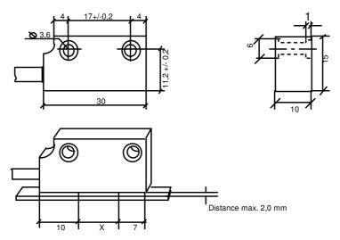
Over the distance X, the gap between sensor and measuring tape must fall between 0,1 and 2,0 mm.
