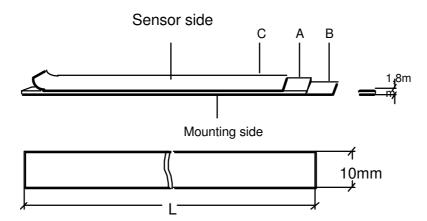
Can be supplied in lengths from 0,5 to 32 m.
