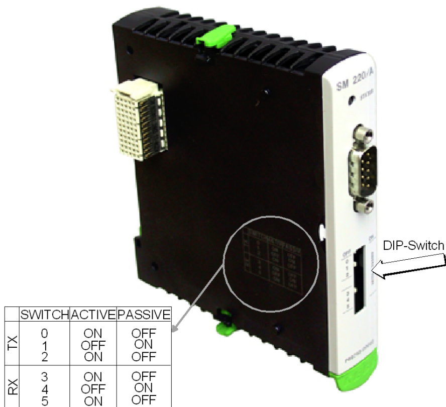
Fig.5-6: Position of the DIP switch and DIP switch position at the SM 220/A
