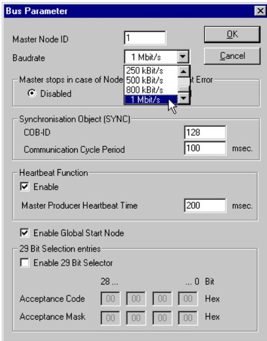
Select the CANopen master and run the "Bus parameters..." command in the "Parameters" menu to set the transmission speed parameter on the CANopen network.
