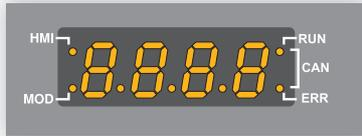
The two LEDs located on the right-hand side of the 7-segment integrated display terminal indicate the CANopen communication status.
