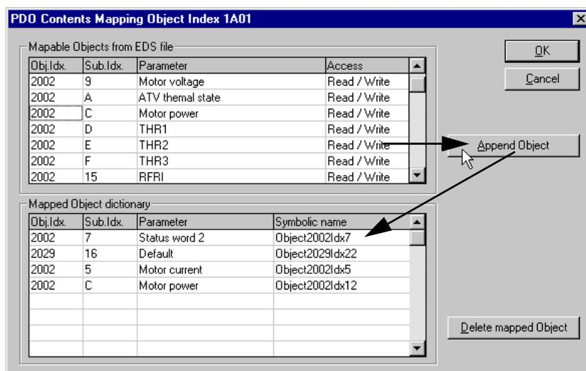
③ **Transmit PDO2:** To configure the assignment of transmit PDO2, select the "Transmit PDO2 parameter" PDO in the "Configured PDOs" section and click the "PDO Contents Mapping" button, or double-click this PDO.
