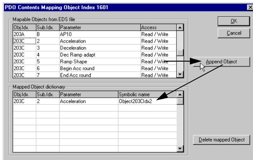
② **Receive PDO2:** To configure the assignment of receive PDO2, select the "Receive PDO2 parameter" PDO in the "Configured PDOs" section and click the "PDO Contents Mapping" button, or double-click this PDO.
