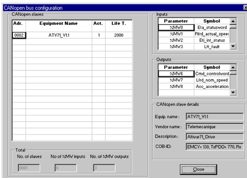
**Note:** These assignments are only valid if the Altiva is the only slave on the CANopen bus and if the two PDOs in sets PDO1 and PDO2 are used as described in the previous example. Configuring other slaves on the same bus or modifying the configuration of the Altivar PDOs will change the assignment of the input and output words described above. In this case, **SyCon** features a command that can be used to view all inputs and outputs: Select "Table Addresses..." in the "View" menu.
