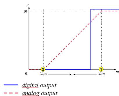
Output in the LIGHT switching mode, analog output in inverse proportionality:
