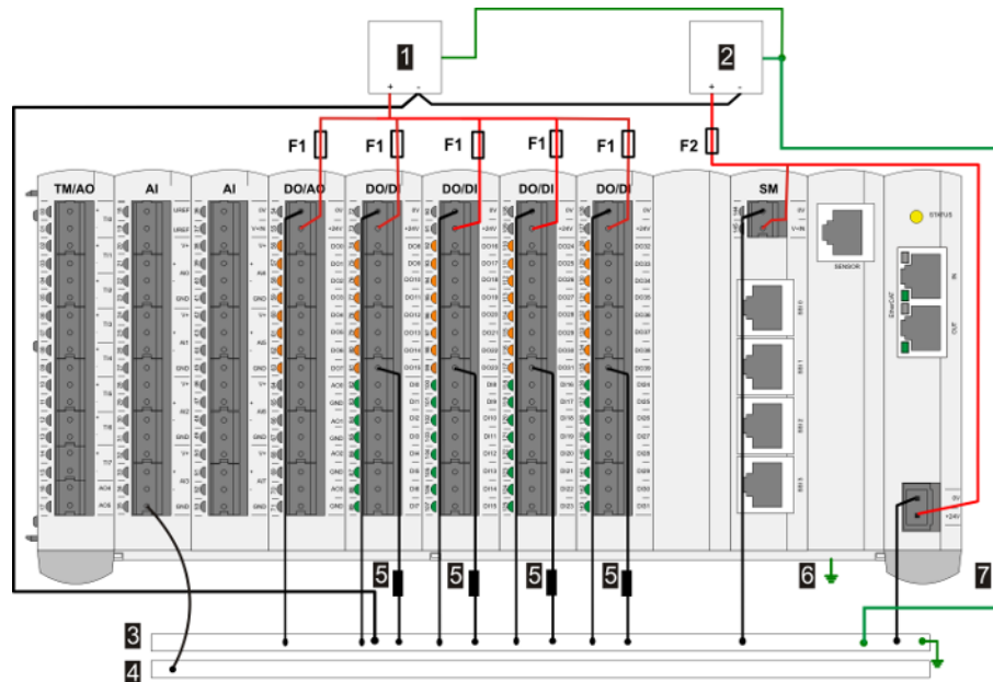
Illustration 6-10: Example: Separate power supply
