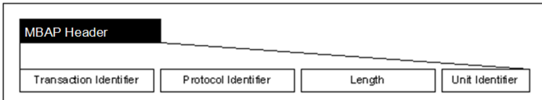
[Figure 5-4] Structure of Modbus TCP/IP ADU
